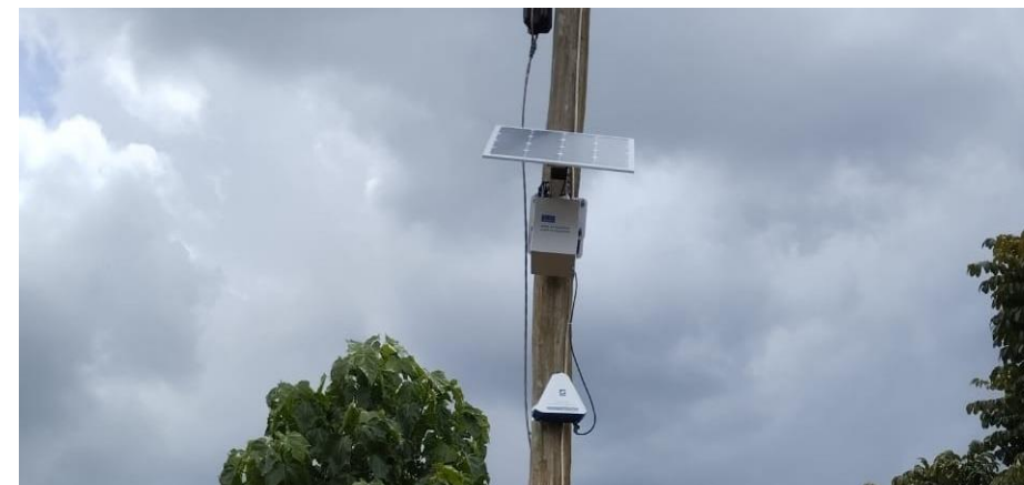
Figure 35 – Air quality sensor installed The Lobo Village in Eldoret (Source: IQAir, https://www.iqair.com/kenya/uasin-gishu/eldoret/the-lobo-village )
