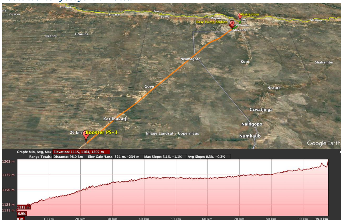
Figure 66. Longitudinal profile of the Section n°2 (S2). Kavango Link-CAN water project. Source: consultant's elaboration using Google Earth Pro data.
