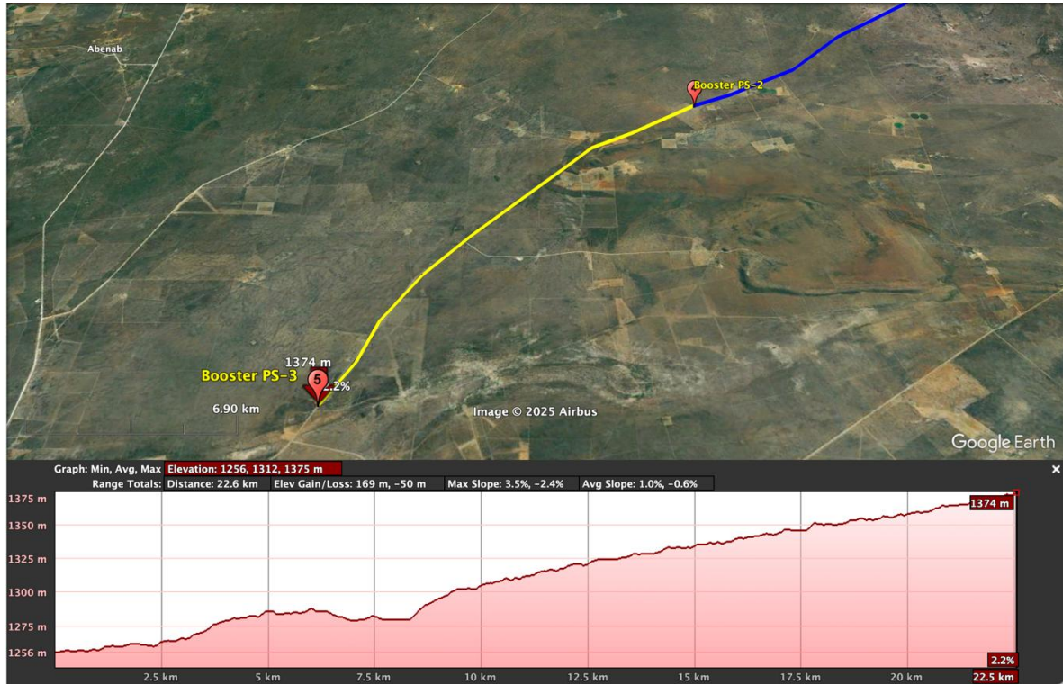
Figure 70. Longitudinal profile of the Section n° 5 (S5). Kavango Link-CAN water project. Source: consultant's Elaboration using Google Earth Pro data.
