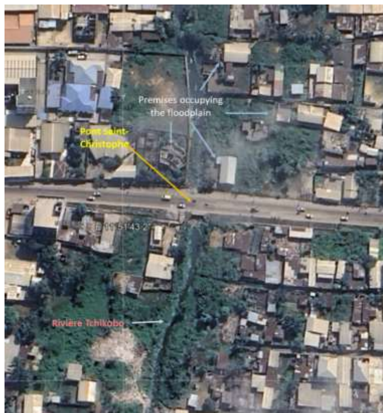
Figure 25. Illustration of the occupation by buildings and premises of the original Tchikobo river floodplain. Source: Authors.
